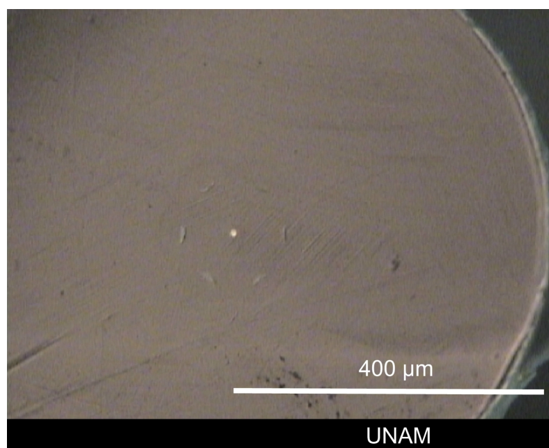
Figure 3.8: Optical microscope image of the fiber after polishing by hand using polishing films.
